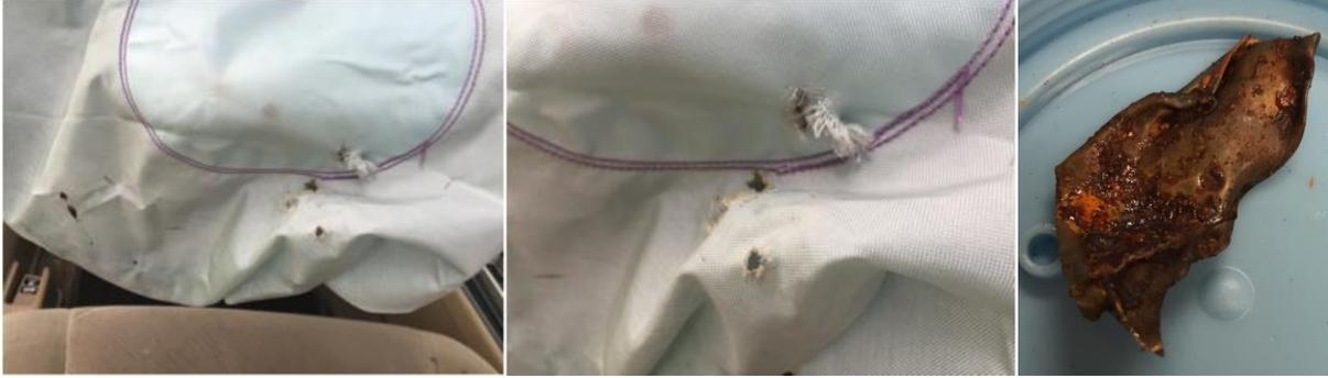
98. Properly designed and manufactured airbag inflators do not explode; instead, they direct the gas and pressure from the burning propellant into the fabric cushion and away from vehicle occupants through vents, inflating the airbag, saving lives, and not peppering vehicle occupants with deadly pieces of shrapnel.
