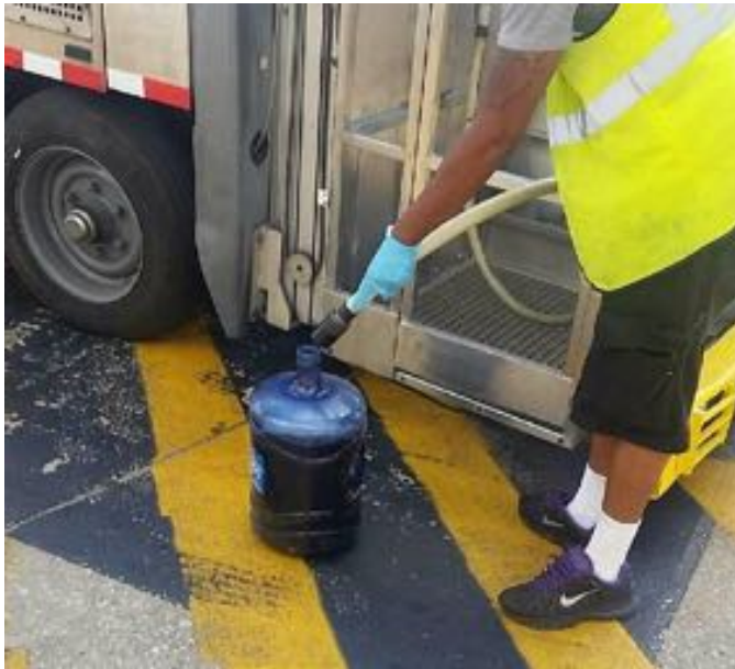
Fig. 3 – An empty Deer Park jug wrongfully taken from a break room at the airport is filled with toxic toilet chemical containing a 6% solution of Bronopol, which is toxic for human consumption, and poisonous to aquatic life. The hose in use is supposed to be attached to the bottom of the plane, and the chemicals are supposed to be filled through a valve on the bottom of the plane, but the valve has been broken for 5 years, and American Airlines has come up with the Deer Park scam to avoid repairing the broken airline parts.
