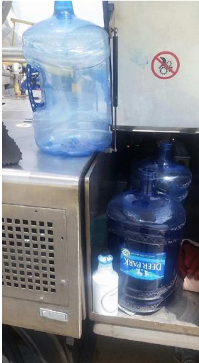
Fig. 4 – Empties carried around in a lavatory truck next to a bottle of poisonous chemical to be used for pouring into the airplane toilets. Not all Lavatory Trucks have compartments like this one. On those trucks lacking compartments, the bottles are carried on the back of the truck. See, e.g., Fig. 9a and 9b, below .
